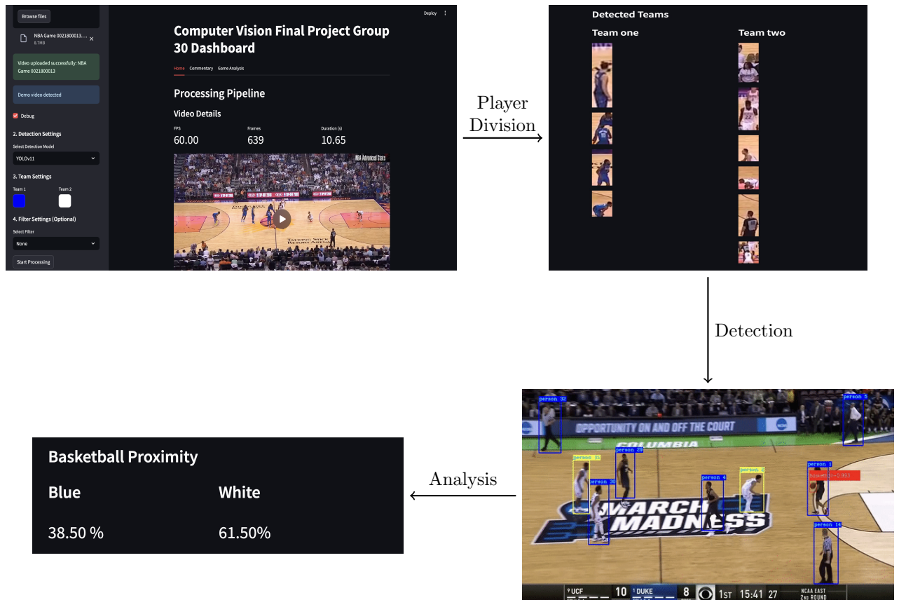
Figure 3: Process flow from manual color selection in the dashboard to detection and analysis results.
